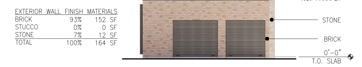
BLDG C EAST ELEVATION SCALE: 3/32" = 1'-0"
